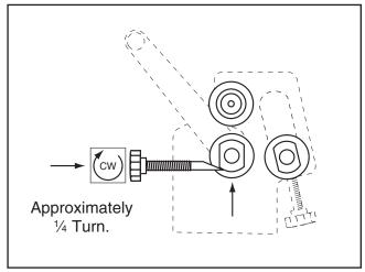
Figure 15. Raising bottom roller <sup>1</sup>/<sub>4</sub> turn.
